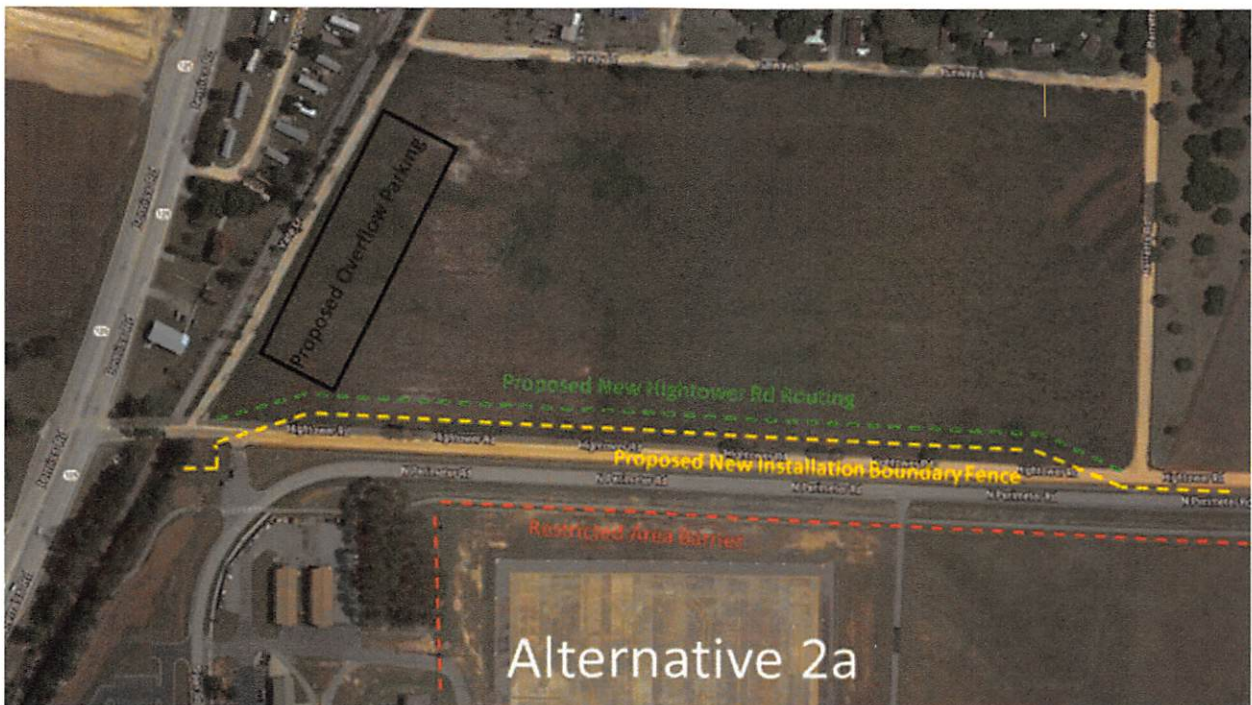
Alternative 2a – Reroute Hightower Road to meet minimum boundary distance requirements
